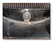
Used to support cracked radiator shells below the crank hole. You can make your own!
