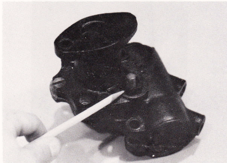
Location of the eccentric for adjustment of proper gear mesh between the sector and the worm.
